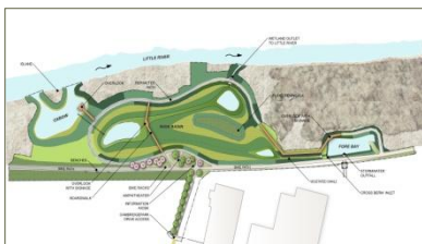
Earthen levees and spillway structures interface with trails, boardwalks, overlooks, an amphitheater, and native plants (trees, shrubs, and wetlands)
