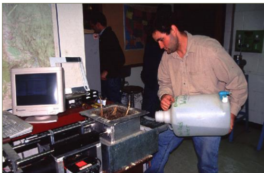
Modified ASTM method direct shear test of saturated vegetated soil allows quantification of root reinforcement
